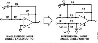
Figure 8. Second-Order Multiple Feedback (MFB) Filter
