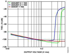
*Figure 10.* THD+N vs.V<sub>OUT</sub> of the ADA4841-2, ADA4807-2, and AD8397
