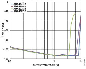
Figure 5. THD + N Result of Recommended Operational Amplifiers
