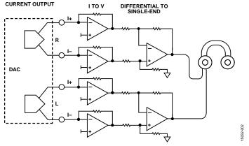
Figure 2. Current Output Configuration
