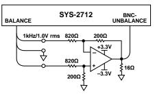
Figure 9. THD + N Test with 16  $\Omega$  Load
