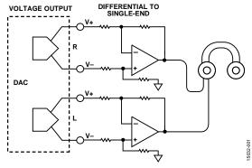
Figure 1. Voltage Output Configuration
