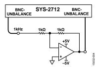
Figure 4. THD + N Test Without Load
