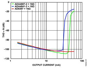
Figure 11. THD+N vs. Iout of the ADA4841-2, ADA4807-2, and AD8397
